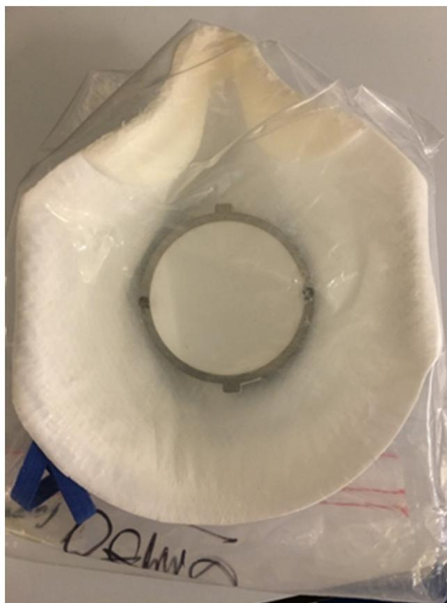
**Figure 1** FFP1 face mask with gelatine filter.
